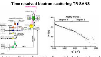
Setup for time resolved Neutron small angle scattering TR-SANS at ILL-D22. The crude liposomes (from fast GPC) with entrapped iron chelate and Boronate are subjected to a pH-jump byfast mixing with a stoppedflow device [5b]. The structure film is collected with logarithmic time scale (5.3 % time increase / frame).
